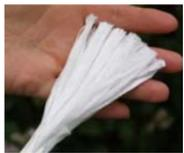
Superwinch/Goodwinch drums have a hole that the end of the rope goes through. Simply cut out 2 of the 12 strands about 10cm/4" from the end, rake out the fibres and tightly bind with insulating tape three or four times so the end is a tight fit to the hole in the drum. Then tighten the grub screw.
