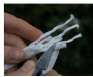
Take the end of the **Dyneema® Bowrope** and cut back 9 of the 12 strands in order to reduce the diameter to form a tapered end which you will then wrap tightly in insulating tape to create an 8cm/3" point.
