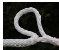
Should you, for whatever reason, be unfortunate enough to cut a **Dyneema® Bowrope** in half, simply cut out the affected area and prepare a pointed 'fid' on each end. Bunch up the 12 strands about 70cm/28" from one end and push the pointed end into the middle and milk it through. Take the other end and do the same but the opposite way. Where the two ends go into the rope you should whip it.
