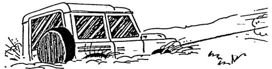
4. After a slight pause, the bogged vehicle is recovered. If the vehicle is not recovered by the first attempt, repeat the process. Once free, continued towing by Recoverline is possible.
